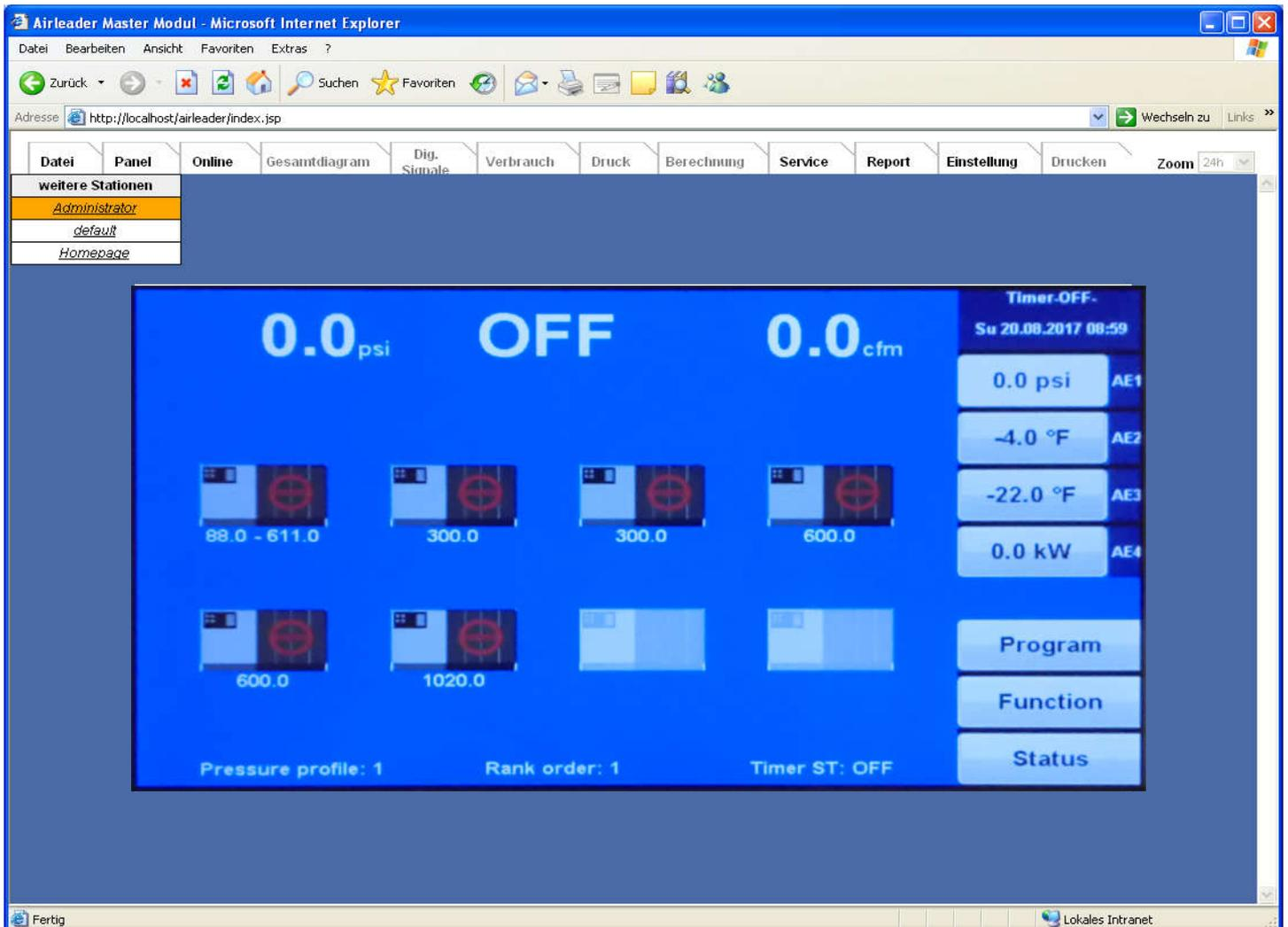
The AIRLEADER Web servers visualization has a card rider system for the basic functions. The possible respectively currently options are active (black dialable), The online visualization shows the status of the compressed air station in real time. Fault or service messages are distributed directly here.
