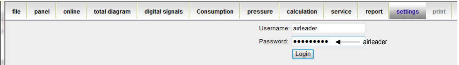
As an introduction to internal settings and remote control of the web server you have to login. On "Settings" - "Login" with the default password "AIRLEADER" for username and password
